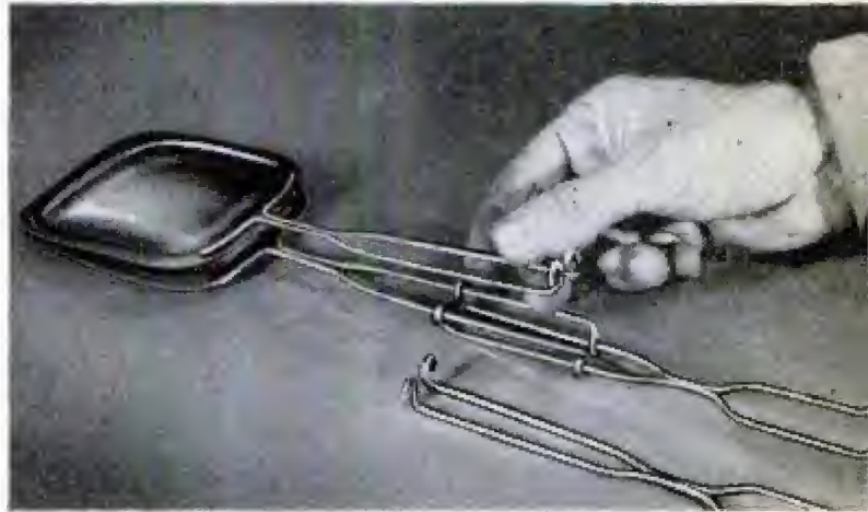
Commercial hamburger grill is used and the handles shortened so that unit can be stored inside the oven
